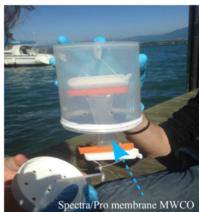
Picture 5: The membrane measurement instrument designed by our research group
